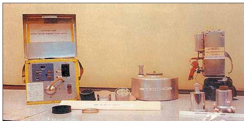
*Radon Monitoring Instrument for Uranium mines/mills*
