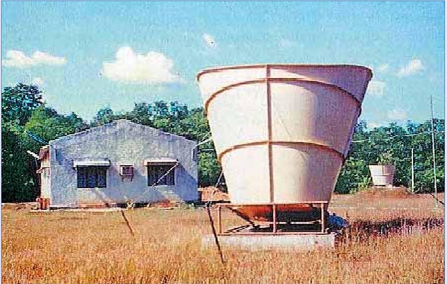
*SODAR equipment at Environmental Survey Laboratory, Kaiga, Karnataka*
