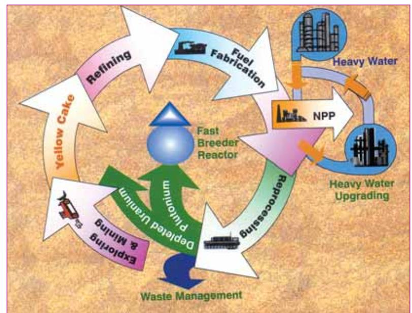
*A pictorial representation of Nuclear Fuel Cycle having a Pressurized Heavy Water Reactor (PHWR) for power generation (shown as NPP)*
