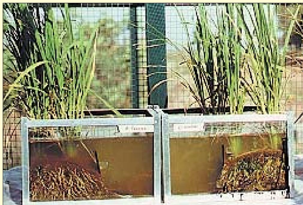
*Continuous flow system developed at BARC to obtain mass balance of carbon-14 labelled pesticides*
