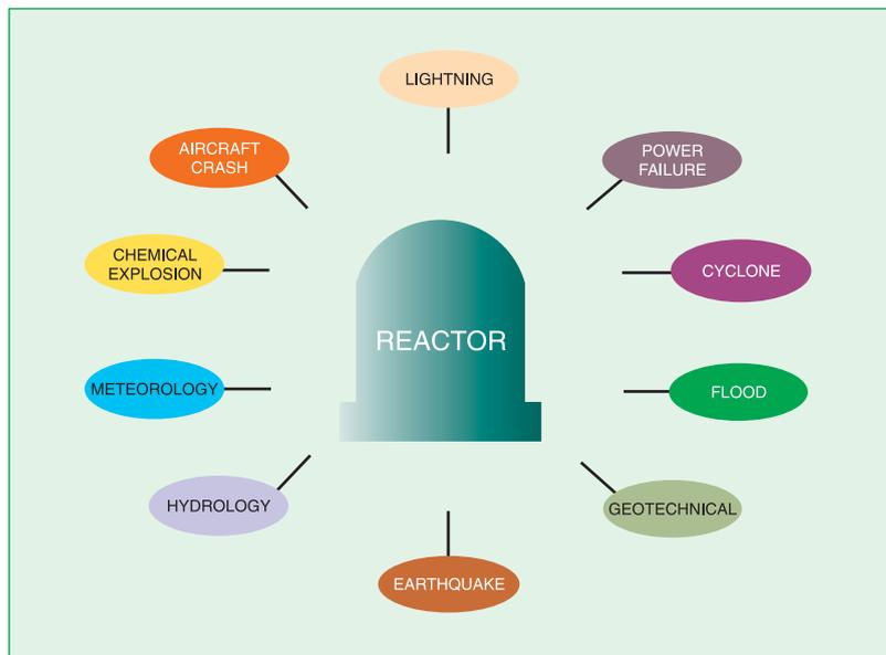
Various external factors to be taken in to account for reactor design (500 MWe PFBR and 1000 MWe VVER reactors) are designed to withstand the earthquake loads expected in the respective regions.
