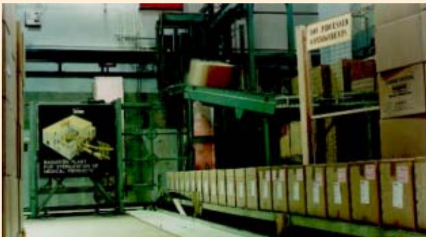
*Medical products sterilized by gamma rays (top) and Isomed plant at Trombay that offers sterilization services to medical industry*
