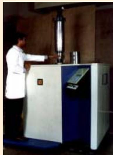
*Gamma chamber irradiator developed by BRIT*
