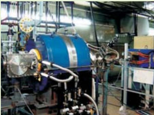
Fig. 2. ECR Ion Source for Radioactive Ion Beam
