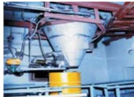
Cementation of sludges using cone mixer assembly at Waste Immobilisation Plant, Trombay
