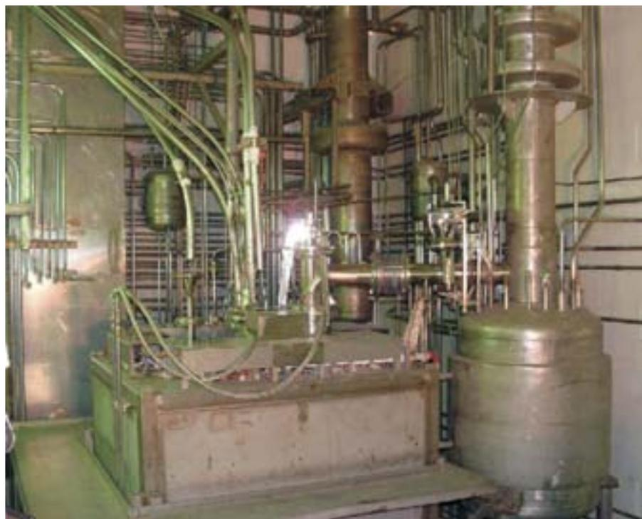
*Joule Heated Ceramic Melter at Advanced Vitrification System, Tarapur*
