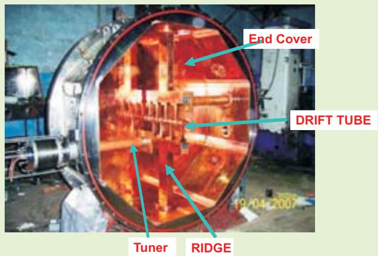
Fig. 5. LINAC during assembly
