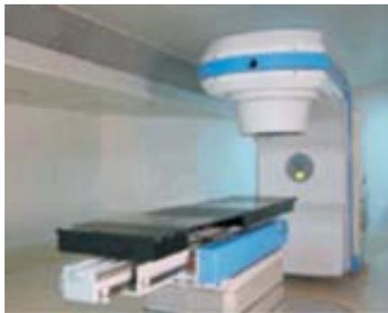
BARC develops indigenous teletherapy machine Bhabhatron that uses Cobalt-60 as radiation source. The machine is commissioned at ACTREC.
