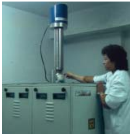
Tissue grafts being irradiated in the Gamma Chamber 1200 in the TMH Tissue Bank.
