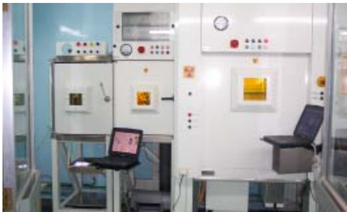
Fully programmable chemistry modules and dispenser used for the synthesis and sterile dispensing of injectable PET radiopharmaceuticals
