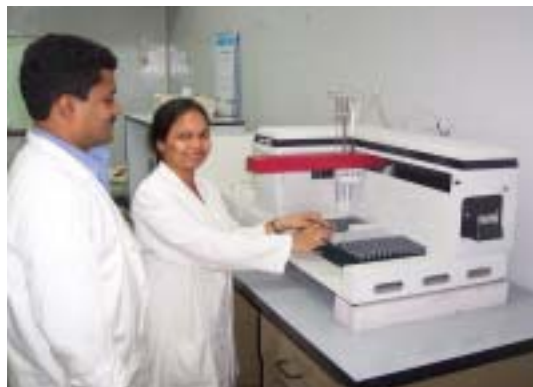
Robotic sample processor for RIA/IRMA that can process samples automatically
