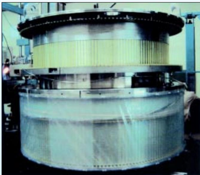
*Superconducting Cyclotron Magnet Coil*
