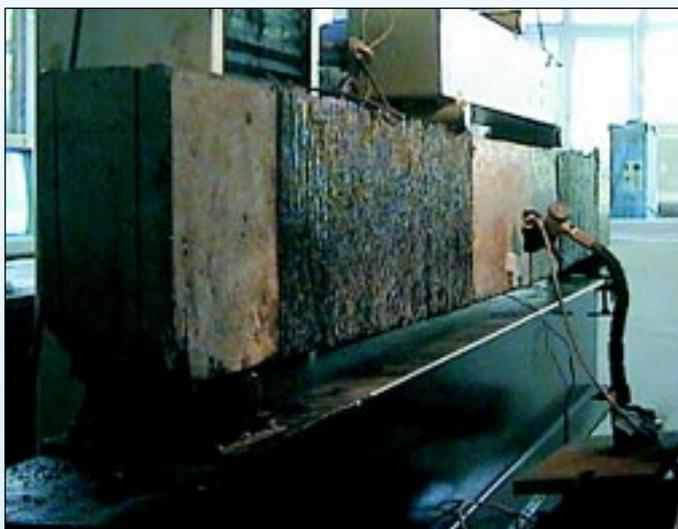
*Testing on flexural elements of Fibre Reinforced Composites, an emerging material for repairing and re-strengthening of the reinforced concrete structures. The project that aims at exploring Fibre Reinforced Composites as retrofitting and repair of reinforced concrete framed structures, is sponsored by DAE.*
