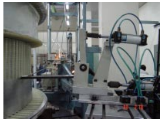
Pressure Arm Assembly guiding the conductor during winding
