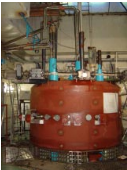
The magnet with the Helium transfer lines
