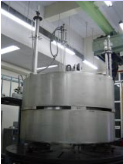
Completed K-500 Superconducting Coil
