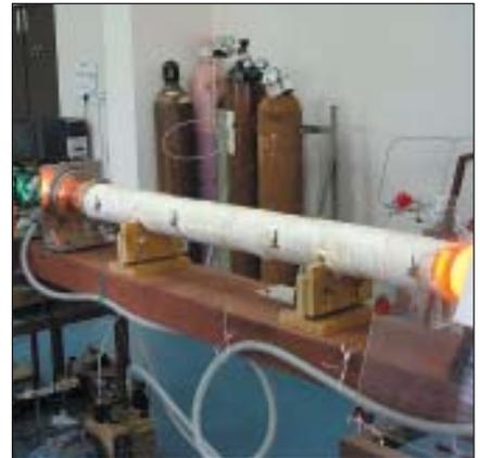
*350 W diode-pumped high power CW IR laser. This laser will be used for various applications in R&D, industry and medicine.*
