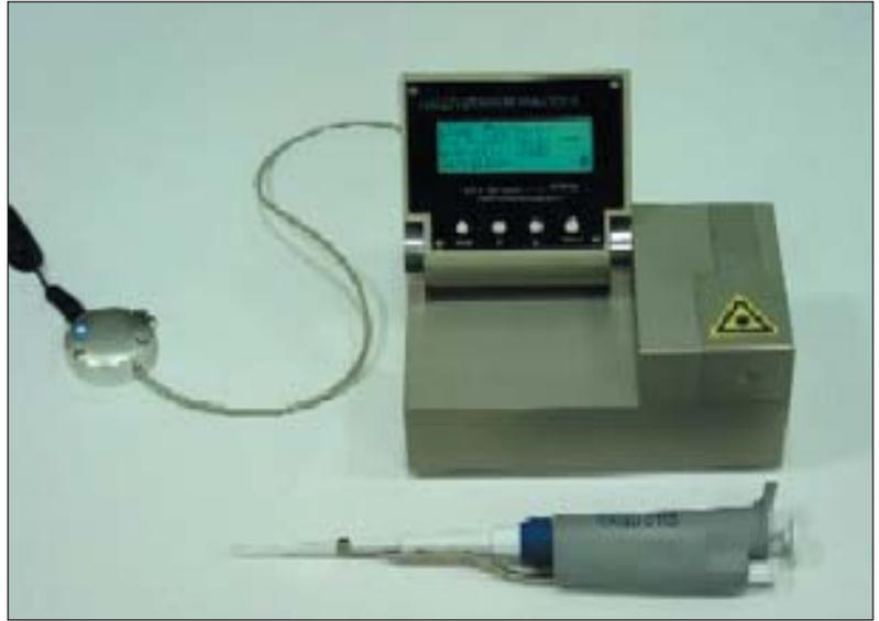
*Laser Uranium Analyser. Twenty such units will be supplied to various units of DAE for uranium mining, radio chemistry, effluent monitoring and health physics applications. Two have been recently supplied to BARC, Mumbai and HWP, Talcher*
