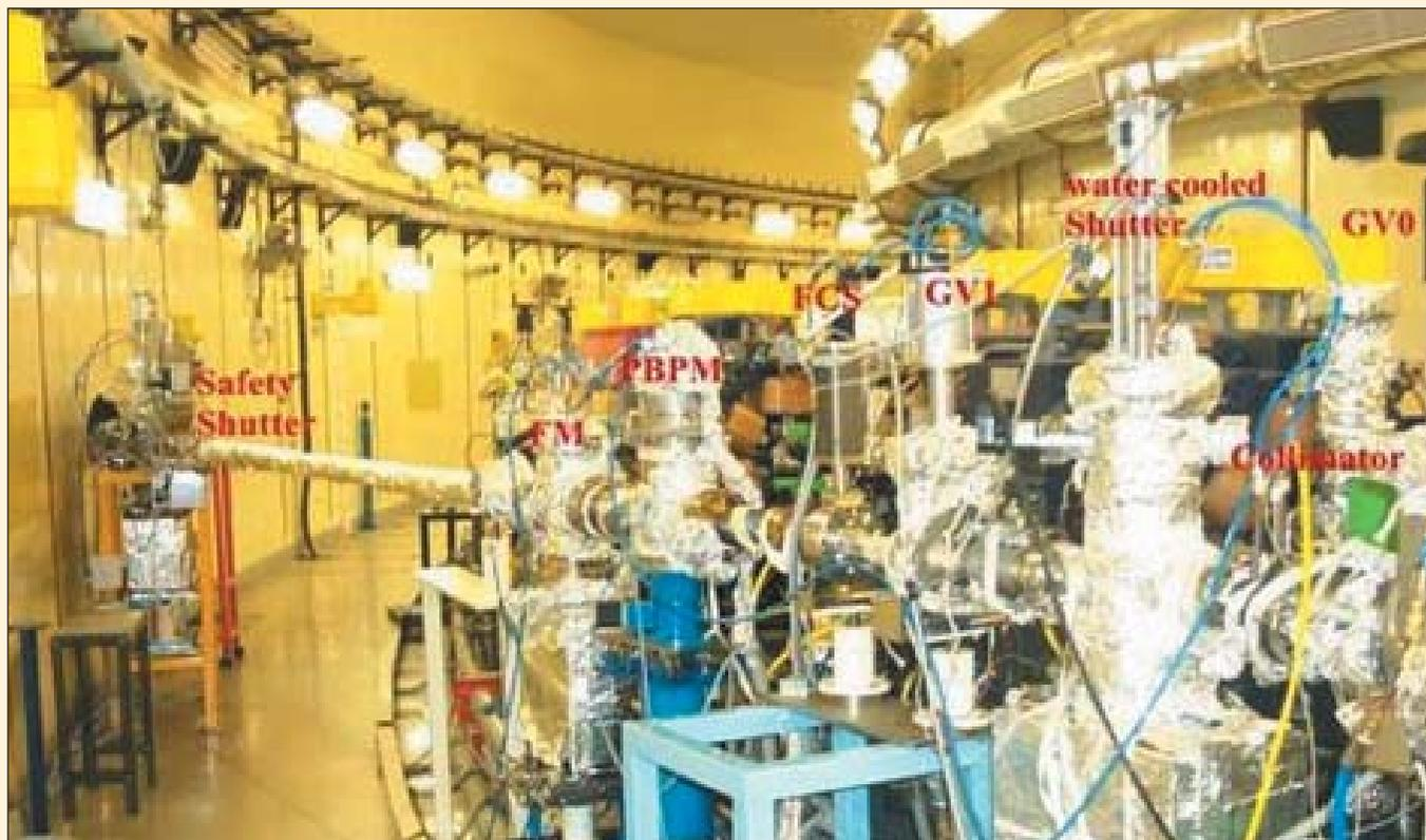
The 2.5 GeV Synchrotron Radiation Source INDUS – II is functioning at Raja Ramanna Centre for Advanced Technology, Indore, Madhya Pradesh. The picture above is of Front-End installed on BL-12, a “High resolution x-ray diffraction beam line” of Indus-2. The Front Ends for five other beam lines, have been taken up for installation.
