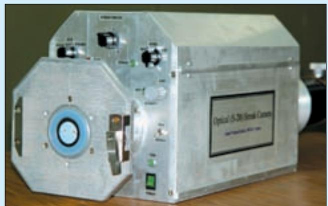
*S-20 optical streak camera developed at RRCAT*
