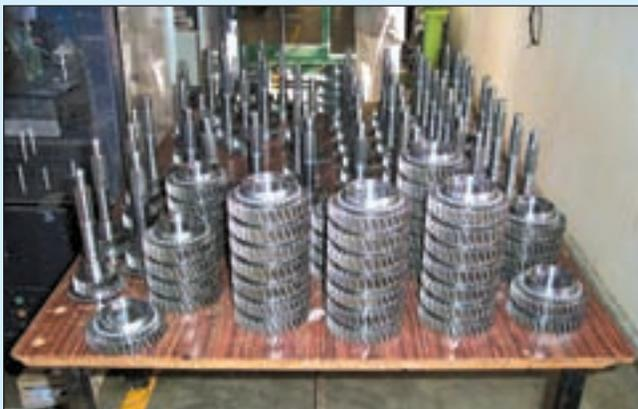
*Laser welded automobile transmission gear assemblies*
