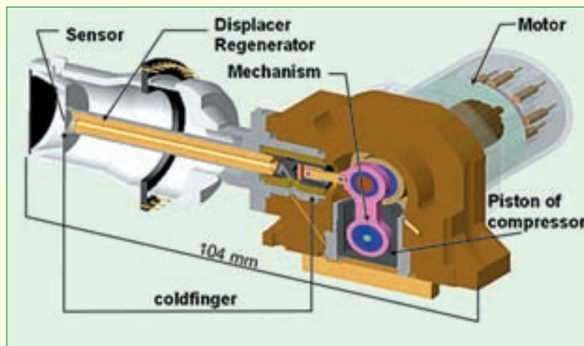
*Schematic of the miniature cryocooler*
