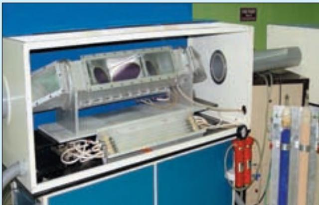
*Nd glass disk amplifier module for high power laser chain developed at RRCAT*
