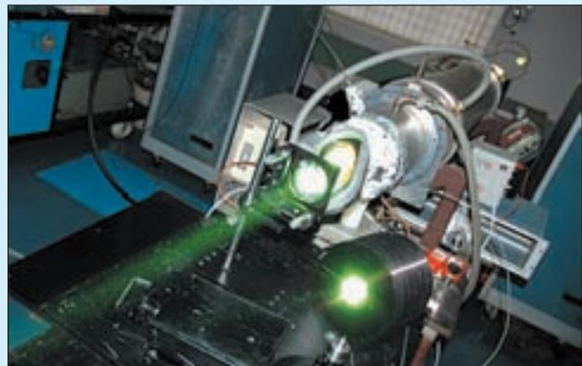
*100 Watt kinetically enhanced copper vapour laser developed at RRCAT*
