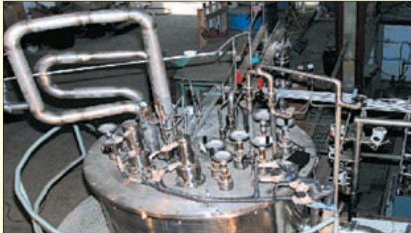
*Helium Refrigerator Cold box showing the turboexpanders, valves and associated piping*
